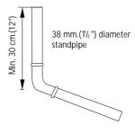
If you intend the drain hose from the machine to empty into a sink, make sure that the sink is empty and the plug hole is not blocked. Use the plastic "U -Piece" supplied.
